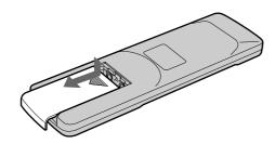
**2** Install two size AA (R6) batteries (supplied) with the correct polarity.
